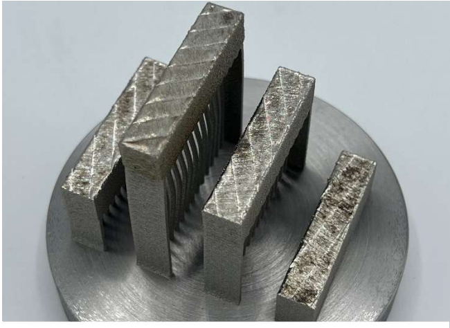
Figure 9: Top surface of specimens manufactured out of Alloy 718 using the original Laser power of 380 W
