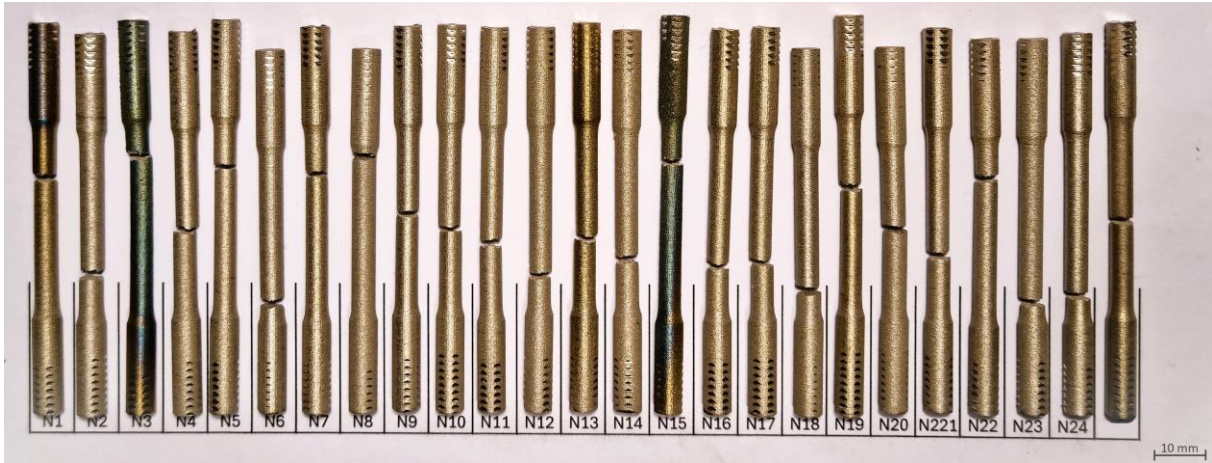
Figure A2: Overview of the tensile specimens after destructive tensile testing, showcasing the breakpoint of each sample; scale: 10 mm.
