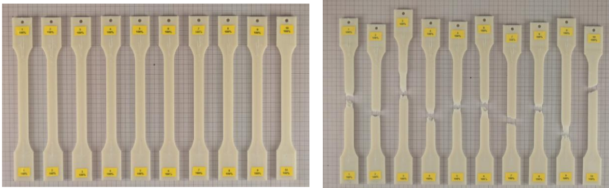
Figure 12: Test specimens before/after tensile testing - Filament 100% flakes content: (a) before (left) and (b) after (right). Picture by the author.
