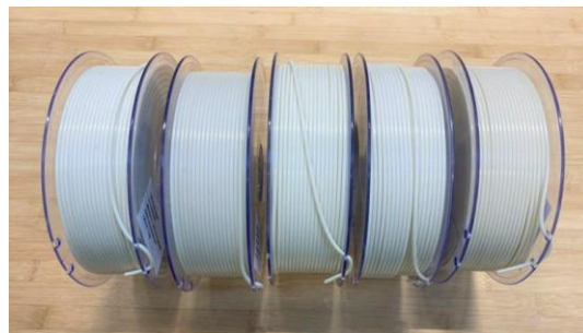
Figure 10: Recycled PA12 filament obtained through Pathways C and D. From right to left there are respectively 100% flakes (no mixing), 90% flakes, 80% flakes, 70% flakes, and 50% flakes. Picture by the author.
