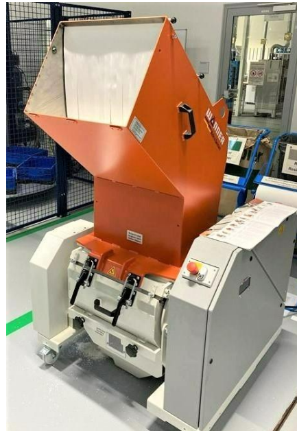
Figure 4: Polymers parts shredder. Picture by the author.
