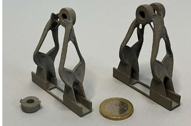
Figure 12: Physical optimized parts after sintering
