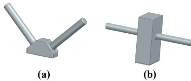
Figure 3: Exemplary CAD-designs of specimens for the preliminary study for (a) 45° angle and (b) 0° angle
