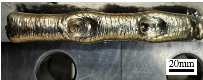
Figure 6: Visualization of the upper process limit due to a centrally split weld seam caused by excessively fast torch movements.
