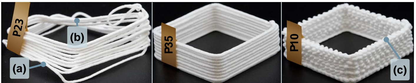
Figure 7: Printed foam test parts of poor (left and right) and good (middle) quality: (a) no print bed adhesion; (b) material carried over due to under-extrusion; (c) material lateral evasion due to over-extrusion
