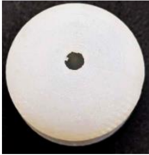
Figure 20: Top view on silicone casting body with hole after decomposition of PVA core in water
