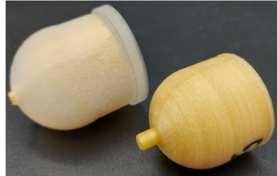
Figure 18: left: Silicone casted part with PVA core, right: PVA core before casting process
