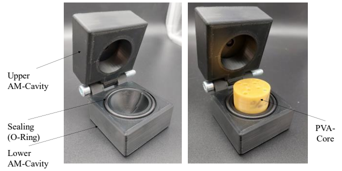
Figure 3: Additively manufactured cavity with additively manufactured PVA core before silicone casting process
