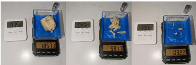
Figure 10: Image sequence of a dissolving PVA core on the precision weight scale
