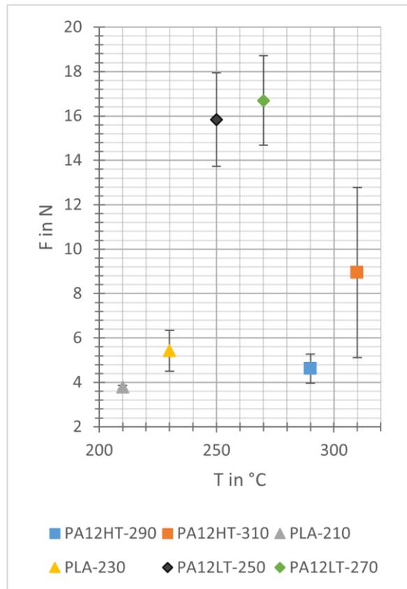
Fig. 4 – Display of mean maximum forces and standard deviations for the maximum holding forces of all measurement series
