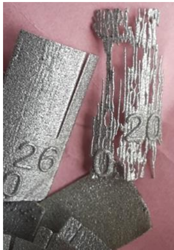
Figure 1: Variants of a simple thin wall object, printed vertically oriented, with various wall thicknesses (constant for each variant): 0,26 mm on the left and 0,20 mm on the right, showing a poor quality where there are partially overlapping offsets in a 316L PBF-LB/M part (the red curve indicates the height of the section visible in Figure 2, located 12 mm above the build plate).
