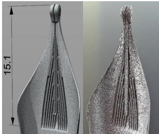
Figure 11: The concave side of the fountain pen nib, including an array of absorptive elements. Left - The mesh output of nTop, rendered in Rhino 5 | Right: The same model, a printed on a Concept Laser M2 Dual Laser Series 3 in Ti6Al4V ELI having 25 \mu\text{m} layers.
