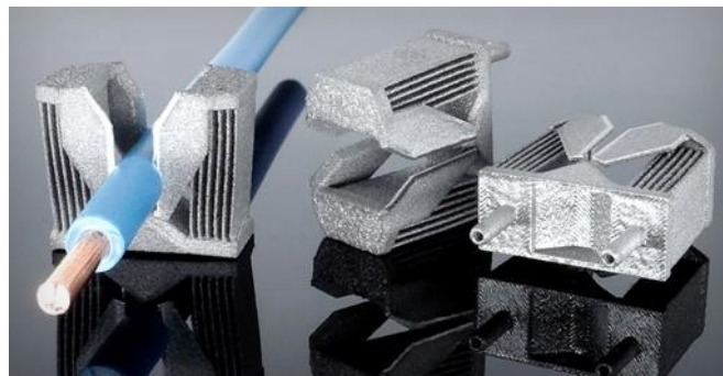
Figure 14: The IDC, in the absence of CuNiSi, printed in Ti6Al4V ELI on a Concept Laser M2 Dual Laser Series 3 having 25 \mu\text{m} layers. The result suggests an effective application of the Scanpath Centric Design method once printed in the intended copper alloy.
