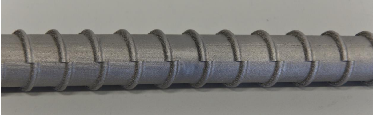
Figure 10: Weld seam on the epee
