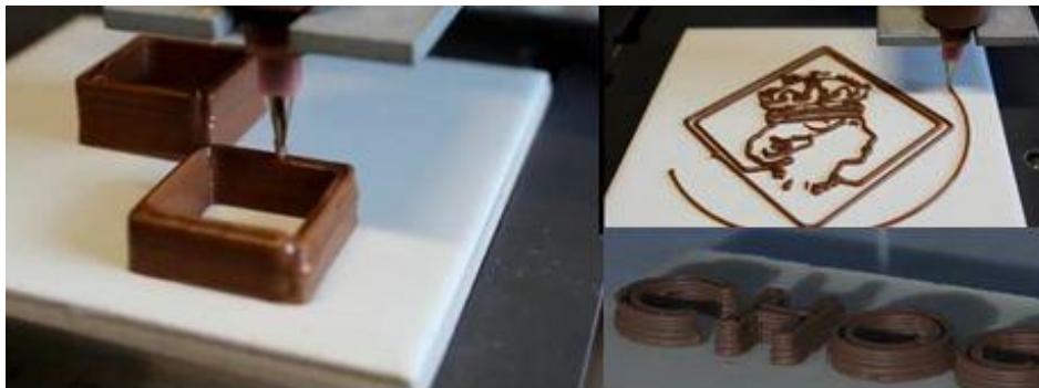
Figure 2: 3D printing of chocolate (3)
