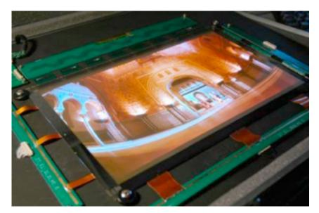
Figure 2: Inkjet printed 14-inch OLED display, by Cambridge Display Technology, U.K. [15]
