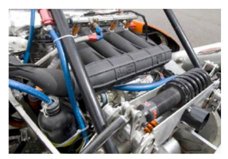
Figure 1: Air intake manifold made using SLS at TNO, the Netherlands [11]
