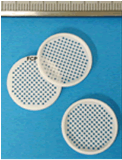
Fig. 23: Grid (sintered alumina)
