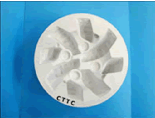
Fig. 12: Deep hole boring head mold (sintered alumina)
