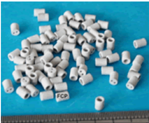
Fig. 25: Electric insulator (sintered aluminium nitride)
