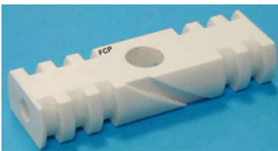
Fig. 18: Core for laser characterisation (sintered zirconia)
