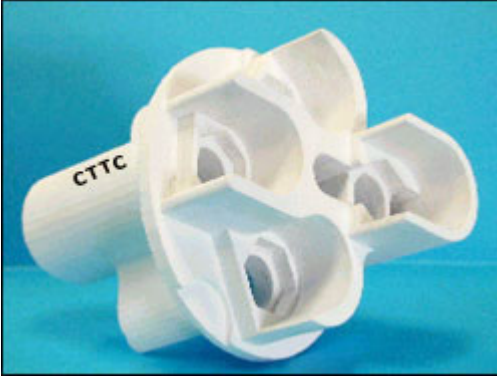
Fig. 11: Connectors (sintered alumina)
