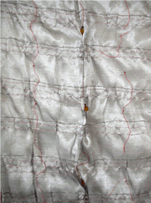
Fig. 5: Sliver – interactive Textile, which is enabled to get in contact with its surrounding due to its ability to emit light signals made by Mette Ramsgrad Thomesn (head of CITA)
