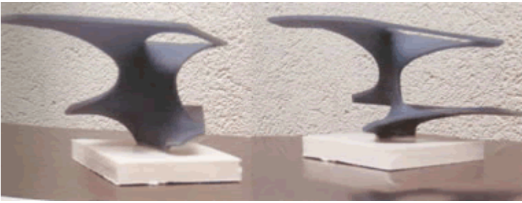
Fig. 2: RP model of the Central Stations main Hub UN-Studio – Ben van Berkel Arnhem Central Station
